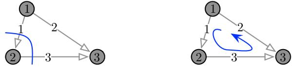
$$\underbrace{\mathbb{R}^m}_{\text{edge space}} = \underbrace{\text{Im}(B^\top)}_{\substack{\text{cutset space} \\ \text{flow vectors}}} \oplus \underbrace{\text{Ker}(B\mathcal{A})}_{\substack{\text{weighted cycle space} \\ \text{cycle vectors}}}$$
