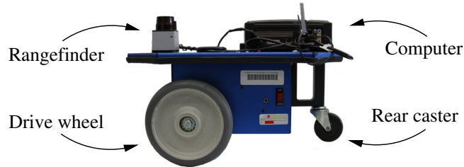
Figure 4.10: Erratic mobile robot with URG-04LX laser rangefinder.
