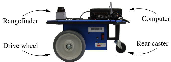
Figure 2.5: Erratic mobile robot with Hokuyo URG-04LX laser rangefinder.
