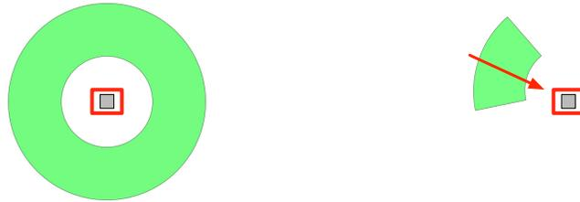
Figure 5.2: Example visibility region  $\text{VIS}_j$  (green shaded area) associated with some target  $T_j$  when  $\text{BEH}_j \neq \text{ANGLE}$  (left), and when  $\text{BEH}_j = \text{ANGLE}$  (right). Notice that the visibility region forms either a full annulus or an annular sector in the ground plane.
