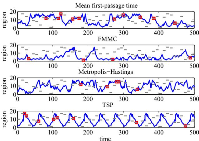
Fig. 5. Performance of mean first-passage time, FMMC, Metropolis-Hastings algorithm and the TSP tour. The solid lines indicate the vehicle trajectory along the graph, gray dots indicate intruder location with time, and the squares indicate intruder detection.
