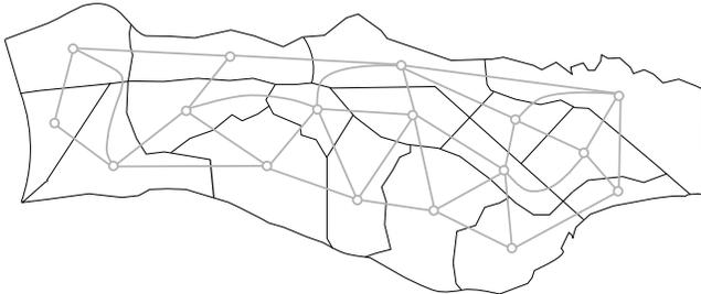
Fig. 4. Environment represented by a doubly-weighted graph. The weight of an edge is its length.
