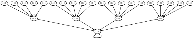
Fig. 3. A subgraph of the transition graph associated with the network matrix A in Example 5. Notice that the sum of the initial states is maintained, and thus average consensus is achieved.
