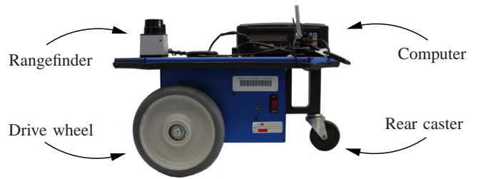
Fig. 6. Erratic mobile robot with URG-04LX laser rangefinder.
