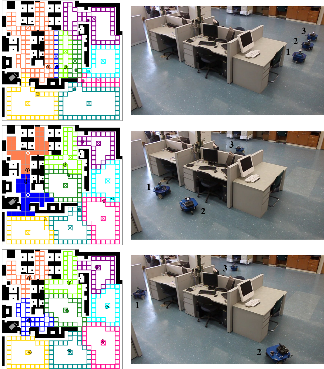
Figure 2.6: Each row contains a territory map and the corresponding overhead camera image for a step of the hardware-in-the-loop simulation. The position of the camera in the environment is shown with a camera icon in the territory map. The physical robots are numbered 1, 2, and 3 and have the orange, blue, and lime green partitions. Their positions in each territory map are indicated with numbered circles.
