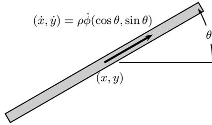
Figure 1.4. Depiction of constraints for rolling disk (the view is from above)
