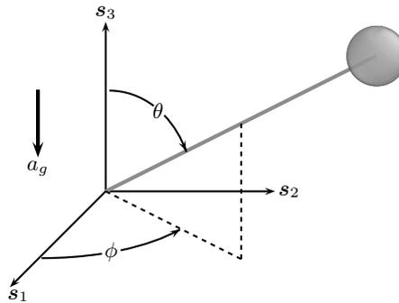
Figure E1.1. Coordinates for spherical pendulum
