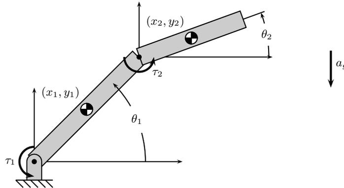
**Figure 1.2.** A two-link planar manipulator
