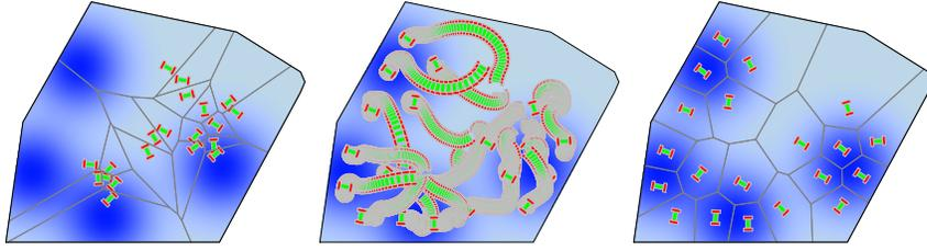
Figure 5.3 Evolution of  $(\mathcal{S}_D, \text{VRN-CNTRD-DYNMCS})$  with  $n = 20$  robots. The feedback gain is  $k_{\text{prop}} = 3.5$ . The left (respectively, right) figure illustrates the initial (respectively, final) locations and Voronoi partition. The central figure illustrates the evolution of the robots. After 20 seconds, the value of the multicenter function  $\mathcal{H}_{\text{distor}}$  has monotonically increased to approximately  $-.555$ .
