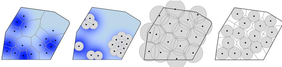
Figure 2.7 From left to right, centroidal,  $r$ -limited centroidal, circumcenter, and incenter Voronoi configurations composed by 16 points in a convex polygon. Darker blue-colored areas correspond to higher values of the density  $\phi$ .
