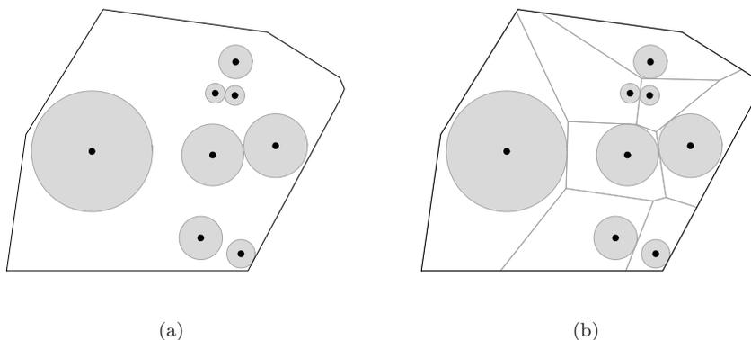
Figure 2.14 Illustration of the definition of  $\mathcal{H}_{sp}$ . (a) and (b) show the same configuration, with and without the Voronoi configuration, respectively. For each node, the disk is the maximum-radius disk centered at the node and contained in the Voronoi cell. The value of  $\mathcal{H}_{sp}$  is the radius shared by the two smallest disks.
