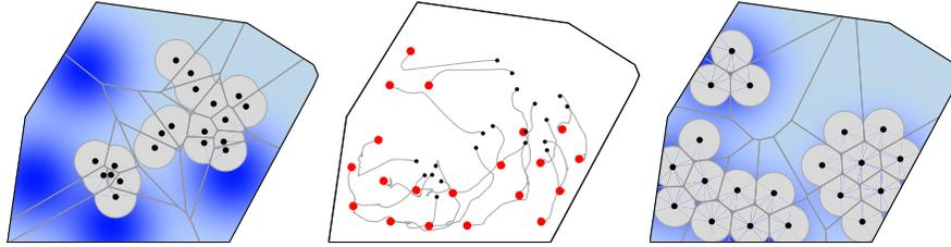
Figure 5.4 Evolution of  $(\mathcal{S}_{LD}, \text{LMTD-VRN-NRML})$  with  $n = 20$  robots and  $r = 0.4$ . The left (respectively, right) figure illustrates the initial (respectively, final) locations and Voronoi partition. The central figure illustrates the evolution of the robots. The  $\frac{r}{2}$ -limited Voronoi cell of each robot is plotted in light gray. After 36 seconds, the value of the multicenter function  $\mathcal{H}_{\text{area}, \frac{r}{2}}$  is approximately 14.141.
