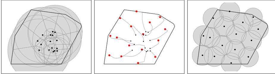
Figure 5.7 Evolution of  $(\mathcal{S}_D, \text{VRN-CRCMCNTR})$  with  $n = 16$  robots. The left (respectively, right) figure illustrates the initial (respectively, final) locations and Voronoi partition. The central figure illustrates the evolution of the robots. After 20 seconds, the value of the multicenter function  $\mathcal{H}_{\text{dc}}$  has monotonically decreased to approximately 0.43273 meters.
