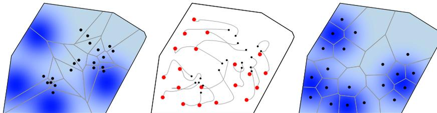
Figure 5.2 Evolution of  $(\mathcal{S}_D, \text{VRN-CNTRD})$  with  $n = 20$  robots. The left (respectively, right) figure illustrates the initial (respectively, final) locations and Voronoi partition. The central figure illustrates the evolution of the robots. After 13 seconds, the value of the multicenter function  $\mathcal{H}_{\text{distor}}$  has monotonically increased to approximately  $-.515$ .
