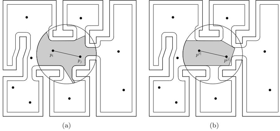
Figure 4.3 The plot in (a) shows the set  $\text{Vi}_{\text{disk}}(p^{[i]}; Q_\delta) \cap \overline{B}(\frac{1}{2}(p^{[i]} + p^{[j]}), \frac{r}{2})$ . The plot in (b) shows the outcome of the execution of the ITERATED TRUNCATION ALGORITHM. Robots  $i$  and  $j$  are constrained to remain inside the shaded region in (b), which is a convex subset of  $Q_\delta$  and of the closed ball with center  $\frac{1}{2}(p^{[i]} + p^{[j]})$  and radius  $\frac{r}{2}$ .
