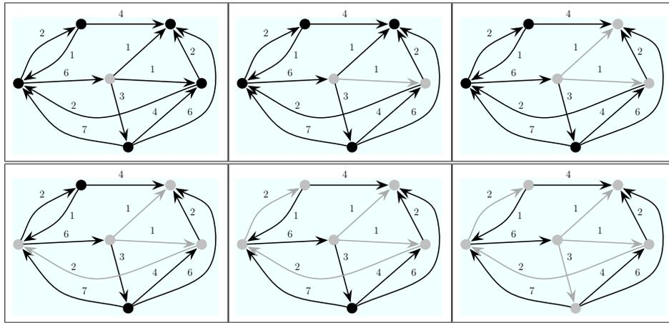
Figure 1.12 Execution of the Dijkstra’s algorithm on the weighted digraph plotted in Figure 1.9. In the top leftmost frame, vertex  $v$  is colored in gray. The other frames correspond to incremental additions of vertices and edges as specified by the function DIJKSTRA. The output of the algorithm is a shortest-paths tree of the digraph rooted at  $v$ . This tree is represented in the last frame with vertices and edges colored in gray.
