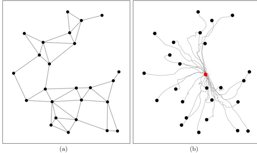
Figure 4.10 Evolution of  $(\mathcal{S}_{\text{LD}}, \text{CIRCUMCENTER})$  with  $n = 25$  robots in 2 dimensions. (a) shows the initial connected network configuration and (b) shows the evolution of the individual agents until rendezvous is achieved.
