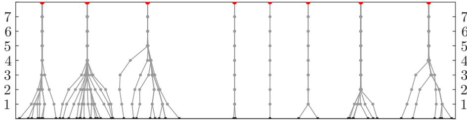
Figure 4.5 Evolution of a robotic network under the AVERAGING control and communication law in Section 4.3.1 implemented over the network  $\mathcal{S}_{\text{disk}}$ , with  $r = 1.5$ . The vertical axis corresponds to the elapsed time, and the horizontal axis to the positions of the agents in the real line. The 51 agents are initially randomly deployed over the interval  $[-15, 15]$ .
