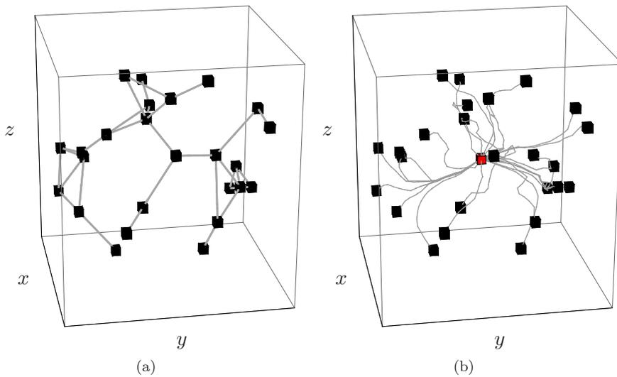
Figure 4.9 Evolution of  $(\mathcal{S}_{\text{disk}}, \text{CIRCUMCENTER})$  with  $n = 25$  robots in 3 dimensions. (a) shows the initial connected network configuration and (b) shows the evolution of the individual agents until rendezvous is achieved.
