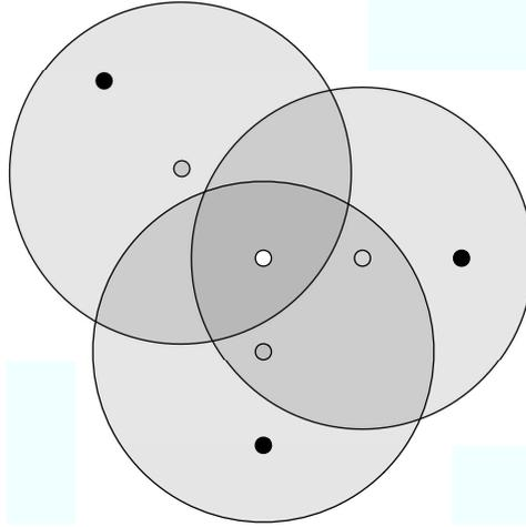
Figure 4.2 Illustration of network connectivity maintenance. The connectivity  $\mathcal{X}_{\text{disk}}$ -constraint set of the white-colored agent is the intersection of the individual constraint sets determined by its neighbors.
