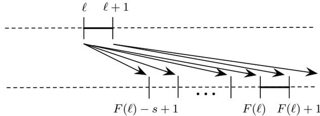
Figure 3.9 Under the rescheduling, the messages that are sent at the time instant  $\ell$  under the control and communication law  $\mathcal{CC}$  are rescheduled to be sent over the time instants  $F(\ell) - s + 1, \dots, F(\ell)$  under the control and communication law  $\mathcal{CC}_{(s, \mathcal{P}_I)}$ .
