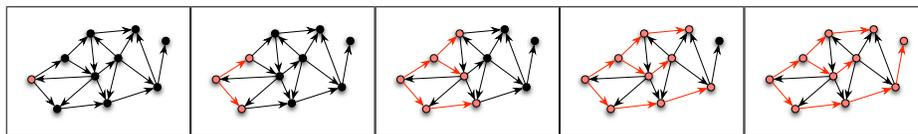
Figure 1.10 Execution of the BFS ALGORITHM. In the leftmost frame, vertex  $v$  is colored in red. The other frames correspond to incremental additions of vertices and edges as specified by the function BFS. The output of the algorithm is a BFS tree of the digraph. The BFS tree is represented in the last frame with vertices and edges colored in red.
