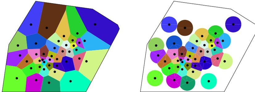
Figure 2.5 Voronoi partition of a convex polygon (left) and  $r$ -limited Voronoi partition inside a convex polygon (right) generated by 40 points. The colored regions correspond to the Voronoi cells and the  $r$ -limited Voronoi cells, respectively, of each individual point.
