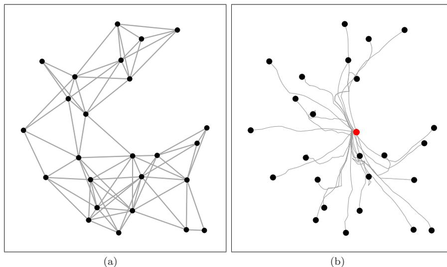
Figure 4.11 Evolution of  $(\mathcal{S}_{\infty\text{-disk}}, \text{PLL-CRCMCNTR})$  with  $n = 25$  robots in 2 dimensions. (a) shows the initial connected network configuration and (b) shows the evolution of the individual agents until rendezvous is achieved.
