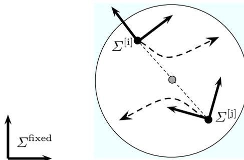
Figure 4.1 Illustration of the connectivity maintenance constraint. Starting from positions  $p^{[i]}$  and  $p^{[j]}$ , the robots are restricted to move inside the disk centered at  $\mathcal{X}_{\text{disk}}(p^{[i]}, p^{[j]}) = \frac{1}{2}(p^{[i]} + p^{[j]})$  with radius  $\frac{r}{2}$ .
