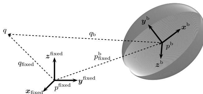
Figure 3.5 Inertially-fixed and body-fixed frames in  $\mathbb{R}^3$
