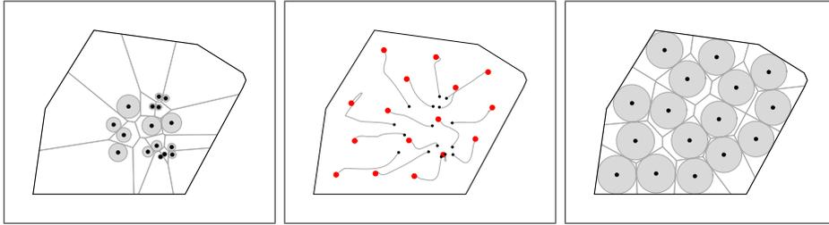
Figure 5.8 Evolution of  $(\mathcal{S}_D, \text{VRN-NCNTR})$  with  $n = 16$  robots. The left (respectively, right) figure illustrates the initial (respectively, final) locations and Voronoi partition. The central figure illustrates the evolution of the robots. After 20 seconds, the value of the multicenter function  $\mathcal{H}_{\text{sp}}$  has monotonically increased to approximately 0.2498 meters.
