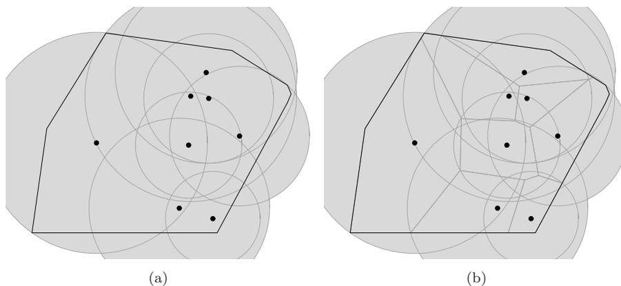
Figure 2.13 Illustration of the definition of  $\mathcal{H}_{\text{dc}}$ . (a) and (b) show the same configuration, with and without the Voronoi configuration, respectively. For each node, the disk is the minimum-radius disk centered at the node and enclosing the Voronoi cell. The value of  $\mathcal{H}_{\text{dc}}$  is the radius of the disk centered at the leftmost node.
