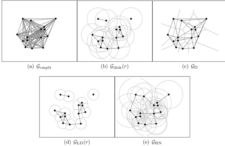
Figure 2.8 Proximity graphs in  $\mathbb{R}^2$ . From left to right, in the first row, complete,  $r$ -disk, and Delaunay, and in the second row,  $r$ -limited Delaunay and relative neighborhood for a set of 15 points. When appropriate, the geometric objects determining the edge relationship are plotted in lighter gray.
