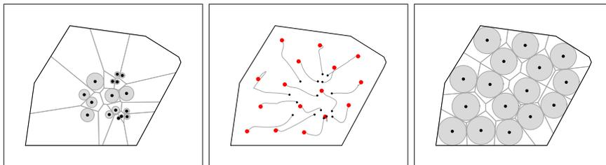
**Fig. 5.8.** Evolution of  $(\mathcal{S}_D, \text{VRN-NCNTR})$  with  $n = 16$  robots. The left (respectively, right) figure illustrates the initial (respectively, final) locations and Voronoi partition. The central figure illustrates the evolution of the robots. After 20 seconds, the value of the multicenter function  $\mathcal{H}_{\text{sp}}$  has monotonically increased to approximately 0.2498 meters.
