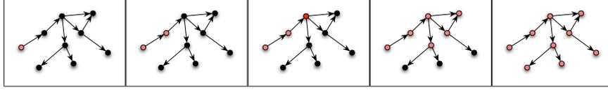
**Fig. 1.12.** Execution of the FLOODMAX algorithm. The diameter of the network is 4. In the leftmost frame, the agent with the maximum UID is colored in red. After 4 communication rounds, its message has been received by all agents.
