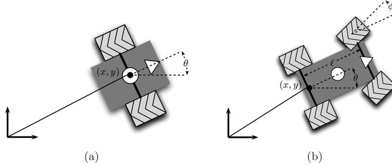
**Fig. 3.1.** (a) Two-wheeled vehicle and (b) four-wheeled vehicle. In each case, the orientation of the vehicle is indicated by the small triangle.
