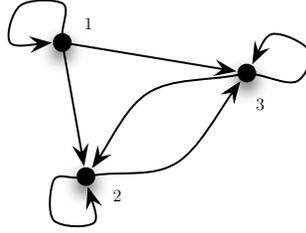
**Fig. 1.10.** Illustration of Proposition 1.29. Even though vertices 2 and 3 are globally reachable, the digraph is not strongly connected because vertex 1 has no in-neighbor other than itself. Therefore, the associated adjacency matrix is reducible.
