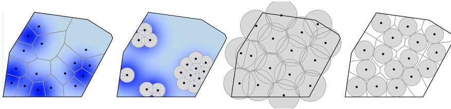
**Fig. 2.7.** From left to right, centroidal,  $r$ -limited centroidal, circumcenter, and incenter Voronoi configurations composed by 16 points in a convex polygon. Darker blue-colored areas correspond to higher values of the density  $\phi$ .
