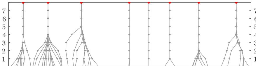
**Fig. 4.5.** Evolution of a robotic network under the AVERAGING control and communication law in Section 4.3.1 implemented over the network  $\mathcal{S}_{\text{disk}}$ , with  $r = 1.5$ . The vertical axis corresponds to the elapsed time, and the horizontal axis to the positions of the agents in the real line. The 51 agents are initially randomly deployed over the interval  $[-15, 15]$ .
