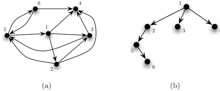
**Fig. 1.11.** Example execution of the FLOODING algorithm. The source is vertex 1. (a) shows the network and (b) shows the BFS tree that results from the execution.
