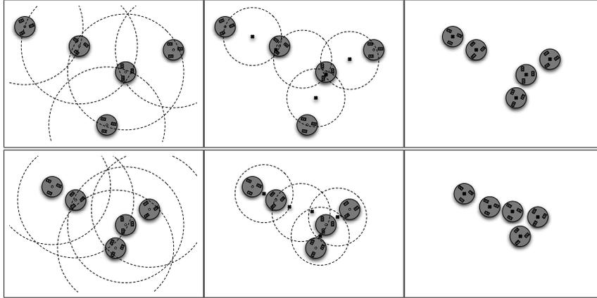
**Fig. 4.6.** Illustration of the execution of CIRCUMCENTER. Each row of plots represents an iteration of the law. At each round, each agent computes its goal point and its constraint set, and then moves towards the goal while remaining in the constraint set.
