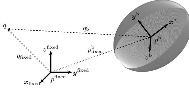
**Fig. 3.4.** Inertially-fixed and body-fixed frames in  $\mathbb{R}^3$
