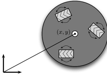
**Fig. 3.2.** Omnidirectional vehicle. In addition to controlling the rotation speed of the wheels, the vehicle can also actuate the direction in which they point. This allows the vehicle to move in any direction according to the first-order dynamics (3.3).
