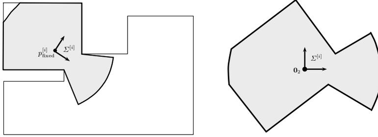
**Fig. 3.6.** The left plot depicts the range-limited visibility set  $V_{\text{disk}}(p_{\text{fixed}}^{[i]}; Q)$  expressed with respect to an inertially fixed frame. The right plot depicts the range-limited visibility set expressed with respect to the body-fixed frame  $\Sigma^{[i]}$ , that is,  $V_{\text{disk}}(\mathbf{0}_2; Q_i)$ .
