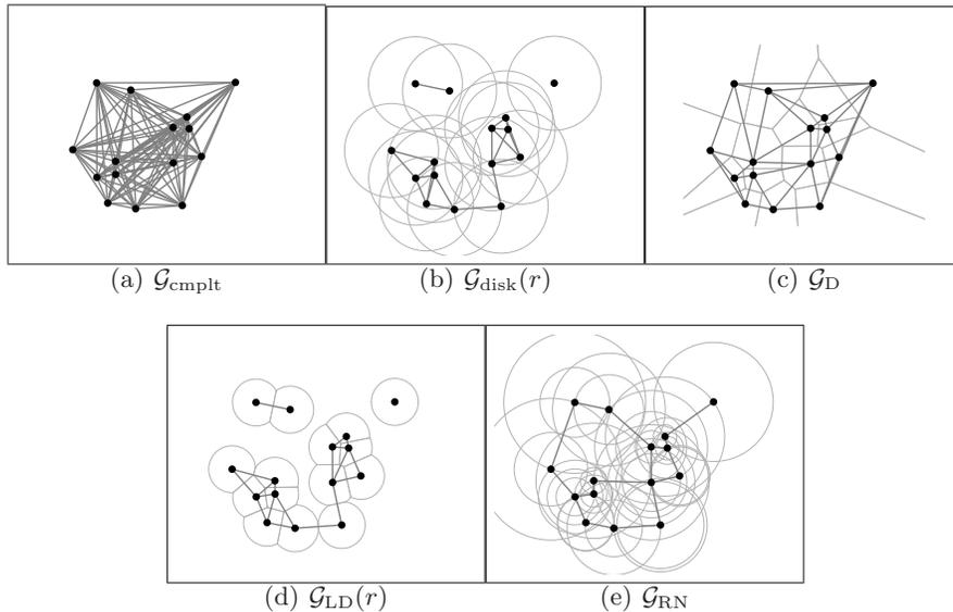
**Fig. 2.8.** Proximity graphs in  $\mathbb{R}^2$ . From left to right, in the first row, complete,  $r$ -disk, and Delaunay, and in the second row,  $r$ -limited Delaunay and relative neighborhood for a set of 15 points. When appropriate, the geometric objects determining the edge relationship are plotted in lighter gray.
