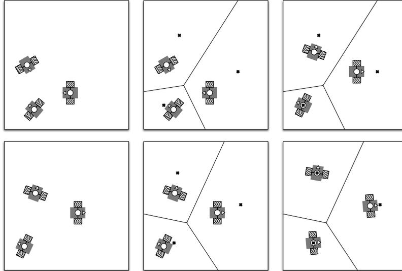
**Fig. 5.1.** Illustration of the execution of VRN-CNTRD-DYNAMCS. Each row of plots represents an iteration of the law. At each round, each agent first computes its Voronoi cell, then determines the centroid, and then moves towards it.
