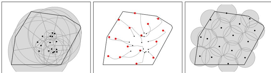
**Fig. 5.7.** Evolution of  $(\mathcal{S}_D, \text{VRN-CRCMCNTR})$  with  $n = 16$  robots. The left (respectively, right) figure illustrates the initial (respectively, final) locations and Voronoi partition. The central figure illustrates the evolution of the robots. After 20 seconds, the value of the multicenter function  $\mathcal{H}_{\text{dc}}$  has monotonically decreased to approximately 0.43273 meters.
