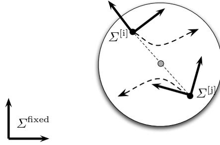
**Fig. 4.1.** Illustration of the connectivity maintenance constraint. Starting from positions  $p^{[i]}$  and  $p^{[j]}$ , the robots are restricted to move inside the disk centered at  $\mathcal{X}_{\text{disk}}(p^{[i]}, p^{[j]}) = \frac{1}{2}(p^{[i]} + p^{[j]})$  with radius  $\frac{r}{2}$ .
