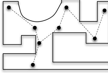
**Fig. 2.11.** Locally-cliqueless graph  $\mathcal{G}_{lc,\mathcal{G}_{vis,Q}}$  of the visibility graph  $\mathcal{G}_{vis,Q}$  for the node configuration shown in Figure 2.9(d).
