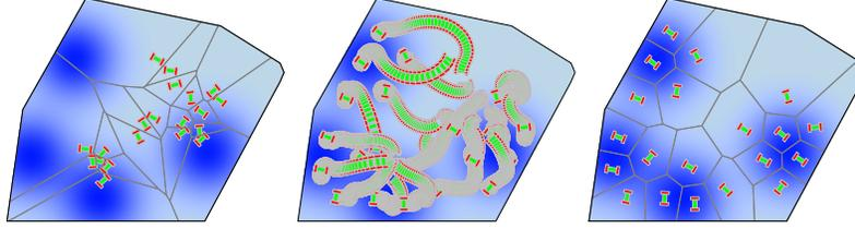
**Fig. 5.3.** Evolution of  $(\mathcal{S}_D, \text{VRN-CNTRD-DYNMCS})$  with  $n = 20$  robots. The feedback gain is  $k_{\text{prop}} = 3.5$ . The left (respectively, right) figure illustrates the initial (respectively, final) locations and Voronoi partition. The central figure illustrates the evolution of the robots. After 20 seconds, the value of the multicenter function  $\mathcal{H}_{\text{distor}}$  has monotonically increased to approximately  $-.555$ .
