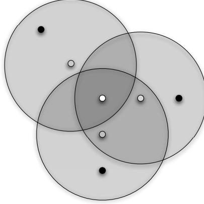
**Fig. 4.2.** Illustration of network connectivity maintenance. The connectivity  $\mathcal{X}_{\text{disk}}$ -constraint set of the white-colored agent is the intersection of the individual constraint sets determined by its neighbors.
