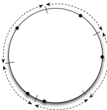
**Fig. 2.6.** Voronoi partition of the circle generated by 5 points. The dashed segments correspond to the Voronoi cells of each individual point.
