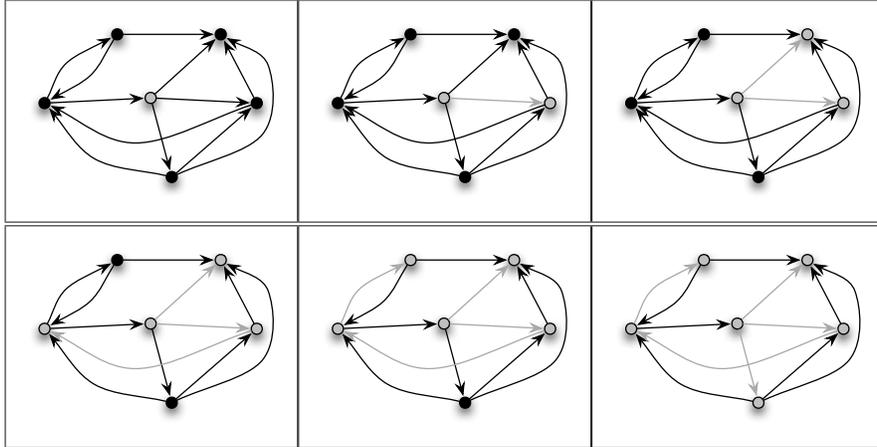
**Fig. 1.9.** Execution of the Dijkstra's algorithm on the weighted digraph plotted in Figure 1.6. In the top leftmost frame, vertex  $v$  is colored in gray. The other frames correspond to incremental additions of vertices and edges as specified by the function DIJKSTRA. The output of the algorithm is a shortest-paths tree of the digraph rooted at  $v$ . This tree is represented in the last frame with vertices and edges colored in gray.
