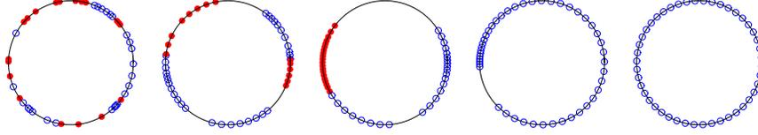
**Fig. 3.3.** The AGREE & PURSUE law. Disks and circles correspond to robots moving counterclockwise and clockwise, respectively. The initial positions and the initial directions of motion are randomly generated. The five pictures depict the network state at times 0, 9, 20, 100, and 800.
