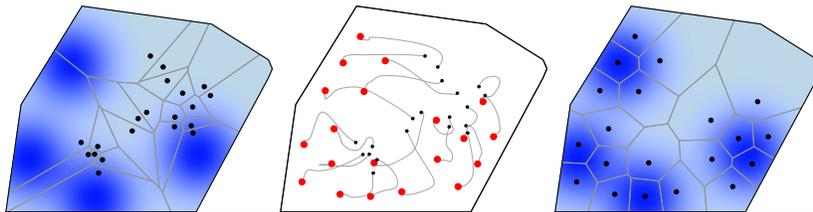
**Fig. 5.2.** Evolution of  $(\mathcal{S}_D, \text{VRN-CNTRD})$  with  $n = 20$  robots. The left (respectively, right) figure illustrates the initial (respectively, final) locations and Voronoi partition. The central figure illustrates the evolution of the robots. After 13 seconds, the value of the multicenter function  $\mathcal{H}_{\text{distor}}$  has monotonically increased to approximately  $-.515$ .
