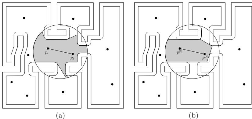
**Fig. 4.3.** The plot in (a) shows the set  $\text{Vi}_{\text{disk}}(p^{[i]}; Q_\delta) \cap \overline{B}(\frac{1}{2}(p^{[i]} + p^{[j]}), \frac{r}{2})$ . The plot in (b) shows the outcome of the execution of the ITERATED TRUNCATION algorithm. Robots  $i$  and  $j$  are constrained to remain inside the shaded region in (b), which is a convex subset of  $Q_\delta$  and of the closed ball with center  $\frac{1}{2}(p^{[i]} + p^{[j]})$  and radius  $\frac{r}{2}$ .
