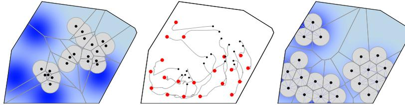
**Fig. 5.4.** Evolution of  $(\mathcal{S}_{LD}, \text{LMTD-VRN-NRML})$  with  $n = 20$  robots and  $r = 0.4$ . The left (respectively, right) figure illustrates the initial (respectively, final) locations and Voronoi partition. The central figure illustrates the evolution of the robots. The  $\frac{r}{2}$ -limited Voronoi cell of each robot is plotted in light gray. After 36 seconds, the value of the multicenter function  $\mathcal{H}_{\text{area}, \frac{r}{2}}$  is approximately 14.141.
