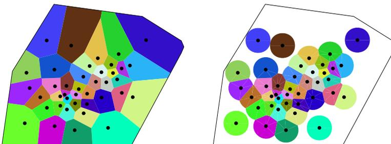
**Fig. 2.5.** Voronoi partition of a convex polygon (left) and  $r$ -limited Voronoi partition inside a convex polygon (right) generated by 40 points. The colored regions correspond to the Voronoi cells and the  $r$ -limited Voronoi cells, respectively, of each individual point.
