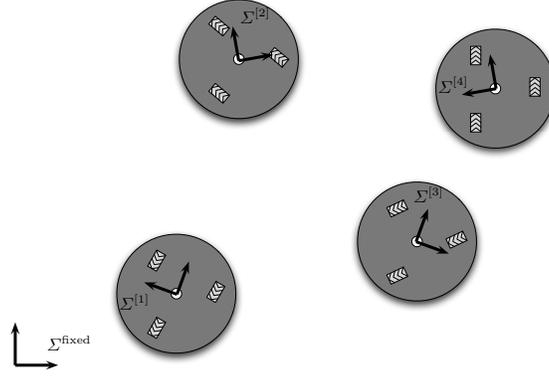
**Fig. 3.5.** Robotic network with relative sensing. A group of 4 robots moves in  $\mathbb{R}^2$ . Each robot  $i \in \{1, \dots, 4\}$  has its own reference frame  $\Sigma^{[i]}$ .
