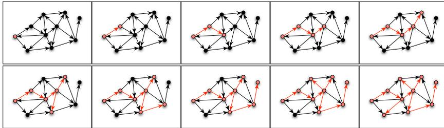
**Fig. 1.8.** Execution of the DFS algorithm. In the top leftmost frame, vertex  $v$  is colored in red. The other frames correspond to incremental additions of vertices and edges as specified by the function DFS. The output of the algorithm is a DFS tree of the digraph. The DFS tree is represented in the last frame with vertices and edges colored in red.
