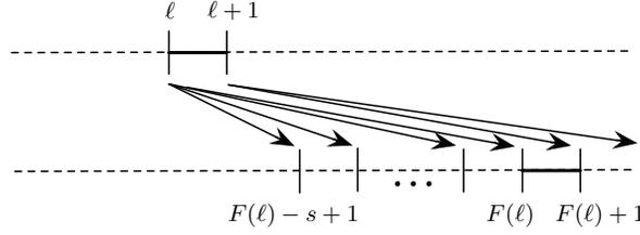
**Fig. 3.7.** Under the rescheduling, the messages that are sent at the time instant  $\ell$  under the control and communication law  $\mathcal{CC}$  are rescheduled to be sent over the time instants  $F(\ell) - s + 1, \dots, F(\ell)$  under the control and communication law  $\mathcal{CC}_{(s, \mathcal{P}_I)}$ .
