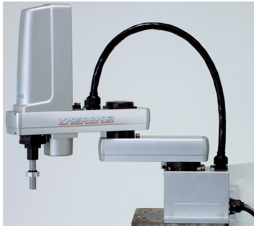
Figure 2.12: The Yamaha© YK500XG is a high-speed SCARA robot with two revolute joints and a vertical prismatic joint. Image courtesy of Yamaha Motor Co., Ltd, http://global.yamaha-motor.com/business/robot .
