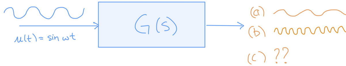
Figure 6.1: System subject to a unit-magnitude sinusoidal input: The main result is that, if the input is a sine wave, so is the output! While the frequency of the output steady state oscillation is the same as the frequency of the input, the magnitude and phase of the output are determined by the frequency response.
