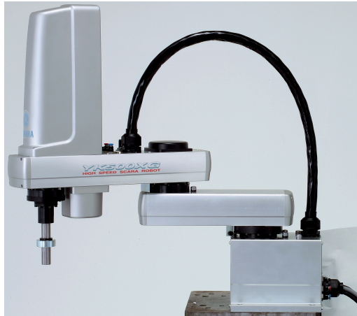
Figure 2.10: The Yamaha© YK500XG is a high-speed SCARA robot with two revolute joints and a vertical prismatic joint. Image courtesy of Yamaha Motor Co., Ltd, http://global.yamaha-motor.com/business/robot .
