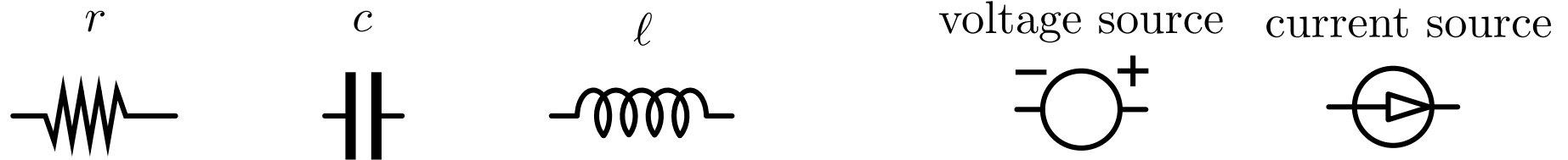
Figure 2.17: Passive elements (resistor, capacitor, and inductor) and active elements (voltage source and current source)
